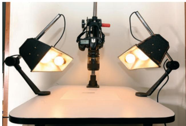
Fig. 1. The digital image analysis system showing specimen position, standardised lighting and camera position.
